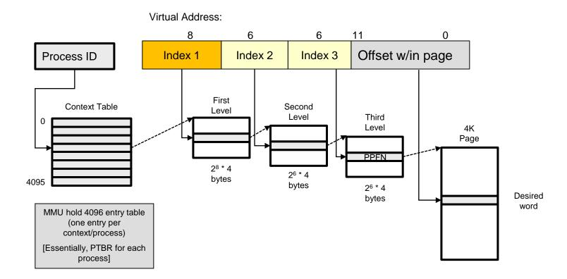
How many accesses to memory does it take to get the desired word that corresponds to the given virtual address? Would that change for a 1- or 2- level table?
