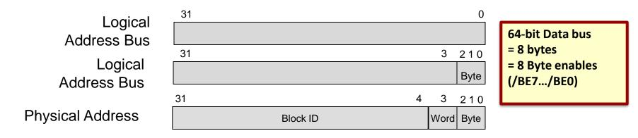
2 Banks so we can quickly get two words to the data cache when a block is transferred
