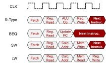
In multi-cycle CPU, each instruction is broken into separate short (and hopefully time-balanced) sub-operations. Each instruction takes only the clock cycles needed, allowing shorter instructions to finish earlier and have the next instruction start.
