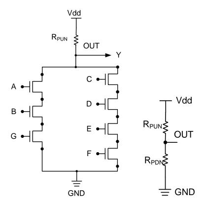
If we model the PUN and PDN as single resistors we can use the voltage divider equation:  $Vout = (R_{PDN} / (R_{PDN} + R_{PUN}))Vdd$
