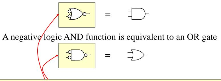
These are the preferred way of showing the N.L. functions because the inversion bubbles explicitly show where N.L. is being converted to P.L. and the basic gate schematics retain their meaning (when we see an AND gate we know we're doing some king of AND function with the bubbles indicating N.L.)
