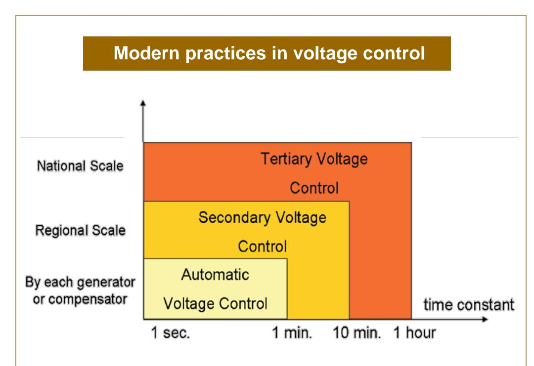
Automatic Voltage Control (AVR): It manages a fast response to fast voltage changes by maintaining the bus voltage at its expected value. It sets the reactive power injection of generators, synchronous condensers, and fast static VAr compensators with the response of 1 ms to 1 min.
