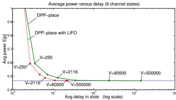
Fig. 10. A comparison of the power-delay tradeoff for DPP-place with and without LIFO. The LIFO data for average delay considers the best 98% of all traffic. Each data point represents a simulation over  $10^6$  slots. Average power is the same for both algorithms whenever  $V$  is the same.
