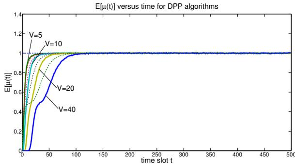
Fig. 5. Average transmission rate  $\mathbb{E}[\mu(t)]$  versus time, obtained from  $10^5$  independent simulation runs over the first 500 slots. The DPP curves are thick, solid, and labeled with  $V \in \{5, 10, 20, 40\}$ . The DPP-place curves are thin dashed curves where  $V \in \{5, 10, 20, 40\}$  corresponds to red, purple, grey, green, respectively.
