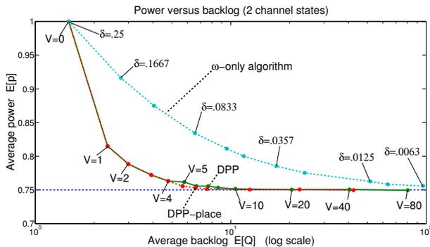
Fig. 4. Average power versus average backlog for the case of 2 channel states. All data points are averages obtained after simulation over 1 million slots. Three algorithms are shown. The drift-plus-penalty (DPP) algorithms use various values of  $V$ . The  $V$  values are labeled for select points on the DPP curve (green). The  $\omega$ -only algorithm uses various values of  $\delta$ .
