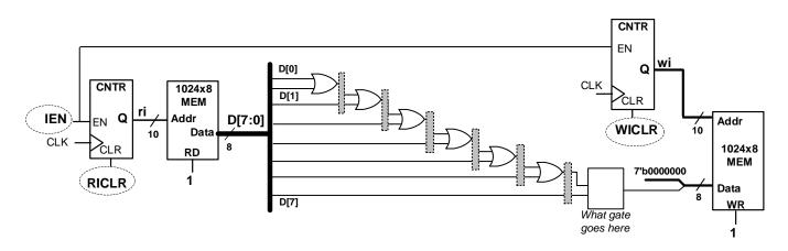
b. Tina Trojan looked at the design and saw some flaws in Billy's pipeline attempt. Without rearranging the OR gates, show where additional pipelining registers are needed by drawing additional shaded rectangles where pipeline registers would be needed.
