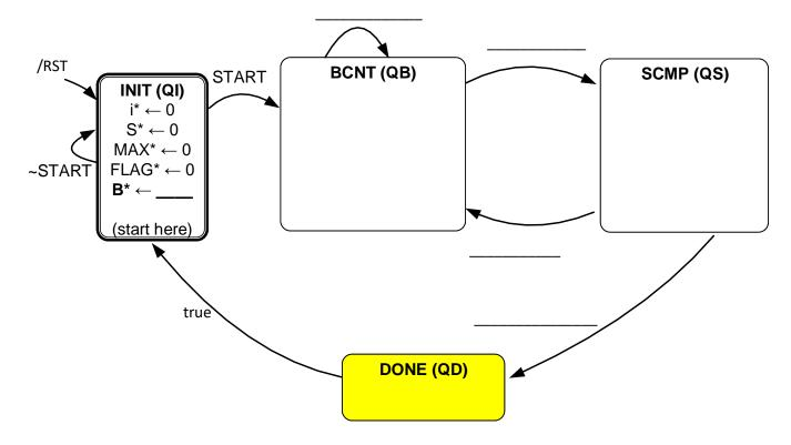
e.) Now suppose we implemented the state machine from the previous part and gave you the one-hot state outputs: QI, QB, QS, and QD. Use these signals plus <u>others that are defined in the datapath</u> to define the control signals indicated below: Just write logic equations using logic operations
