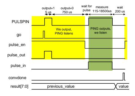
**3. Starting our Design:** The major task in this design is to produce a signal for a given period time. To do this we must know our clock frequency. In the block
