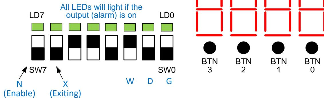
Figure 1 - Switches will be used as the eNable, eXiting, and Windows, Door, Garage sensor inputs. All the LEDs will light up if the Alarm output is 1 (on). The 7-segment displays and buttons will not be used.
