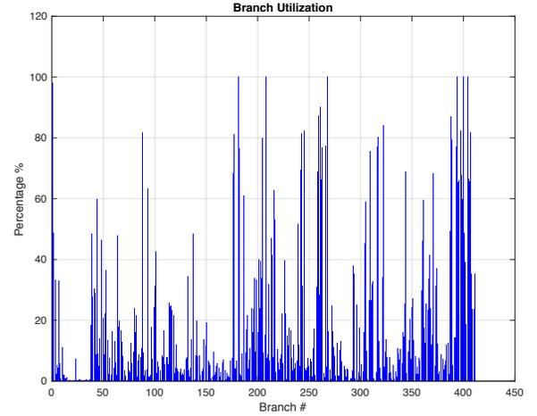
Fig. 5. Utilization Factor ( $\mu_{AC}$ ) for the AC model of the IEEE300 bus system with ORC-OPF implementations and a 700 MW active power constraint
