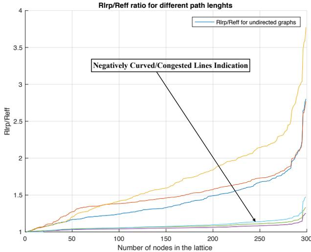
Fig. 1. Flat areas of  $\rho_{lrp}/\rho_{eff}$  curves for the  $P$ -graph of the IEEE300 bus system indicating negative curvature along the corresponding paths
