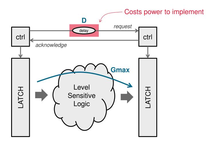
**Gmax < D** Hard to "sign-off" across different process corner, voltage, temperature
