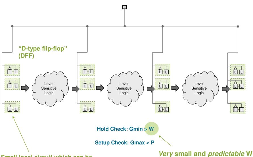
Small local circuit which can be carefully crafted and characterized across multiple process corners, voltages, temperatures
