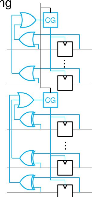
Some parts of register may stay at logic 0 more than logic 1
