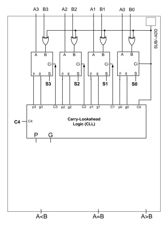
3.2. (5 + 5 + 5)Design a 4-bit comparator to compare two 4-bit SIGNED numbers X[3:0] and Y[3:0] using a 4-bit adder-subtractor given below and additional gates as needed. Hint: Consider the overflow in *signed* subtraction (as the MIPS SLT instruction might do) [You may not have covered the MIPS instruction set yet, in which case you can ignore the parenthetical comment].
