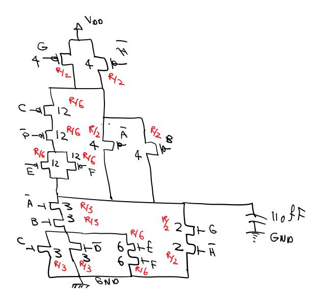
b) In the worst case only path is ON. However the way we have sized each path is to match the current drive of a reference Inverter, i.e., for each path the equivalent resistance is the same as the resistance of the reference Inverter:
