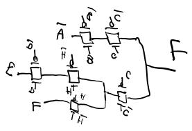
(b) To do the design using NMOS pass transistors only, we would remove all the PMOS transistors. Since all the transistors have the same size of W, then we would save half of the area:
